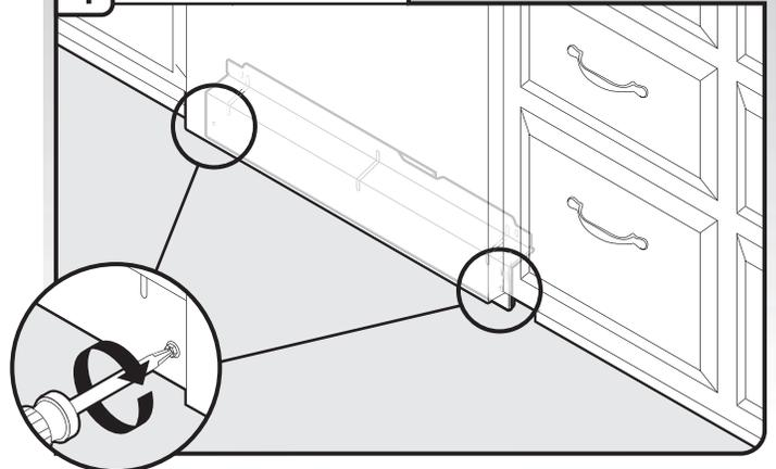
Tighten access panel screws.
